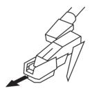
Untie the FM antenna and allow it to hang down in a straight line for optimum FM reception. If you have trouble tuning in an FM station, move the external FM antenna for best reception. Do no connect FM antenna to outside antenna.
